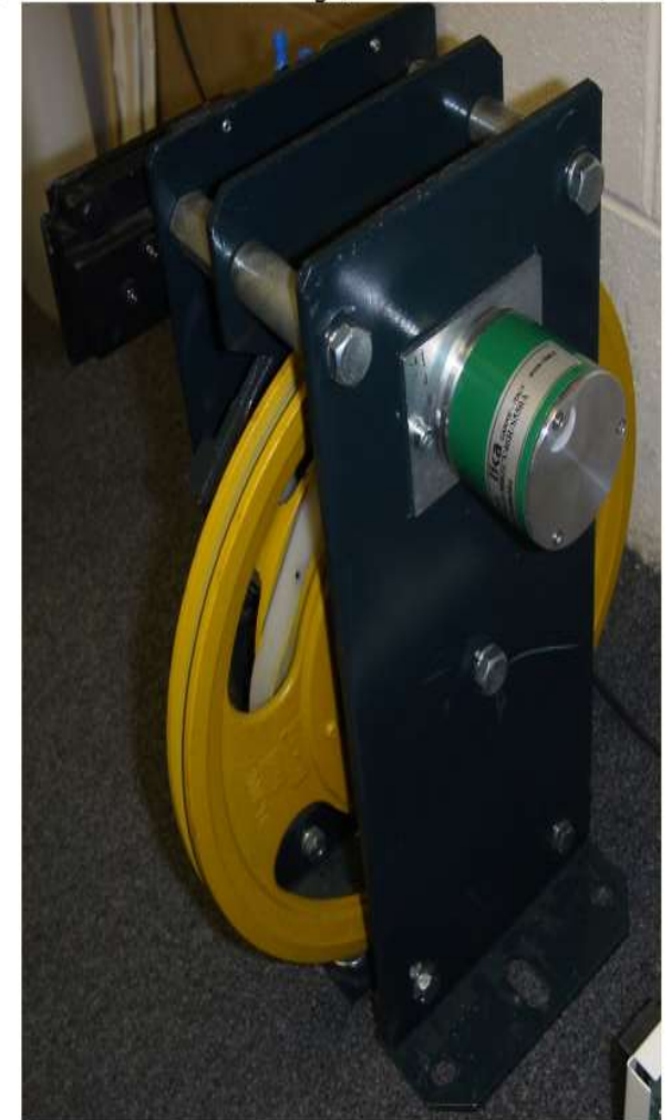
Overspeed Governor with Encoder Mounting (6mm Shaft Encoder)
